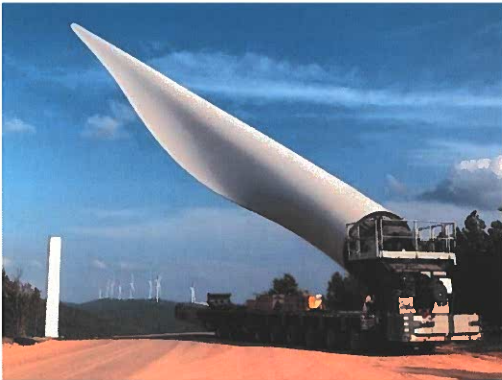
Figure 1.3.3c - Goldhofer Blade Transport Vehicle
